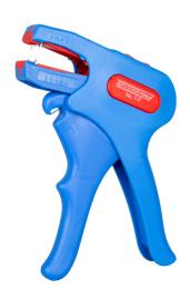
The WEICON Wire Stripper No. 7-F is particularly suitable for 2- or 3-core PVC-insulated flat cables from 0.75 - 4.0 mm². The tool offers a fine-tuning mechanism, which can be adjusted to various positions. The stripping tool has a visual length scale from 8 - 24mm. A well-accessible side cutter is integrated in the tool, which is suitable for cable diameters up to 3 mm and has replaceable blades.
